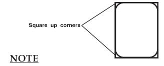
It may be necessary to slightly modify the switch opening to allow the new Switch to be inserted in place. Use a metal file to square up the corners of the switch opening as shown.
